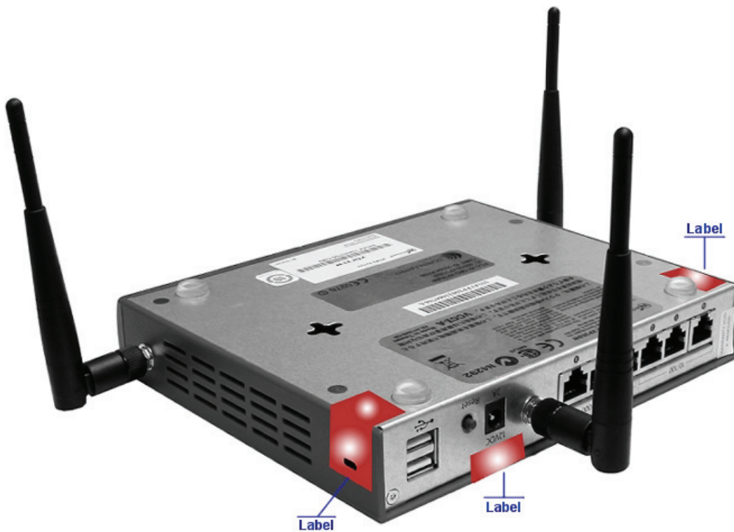
Figure 3: WatchGuard XTM 21/22/23 Wireless Tamper Evident Label Placement
