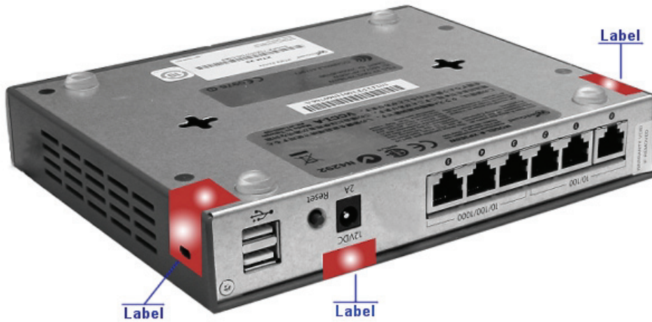
Figure 2: WatchGuard XTM 21/22/23 Tamper Evident Label Placement
